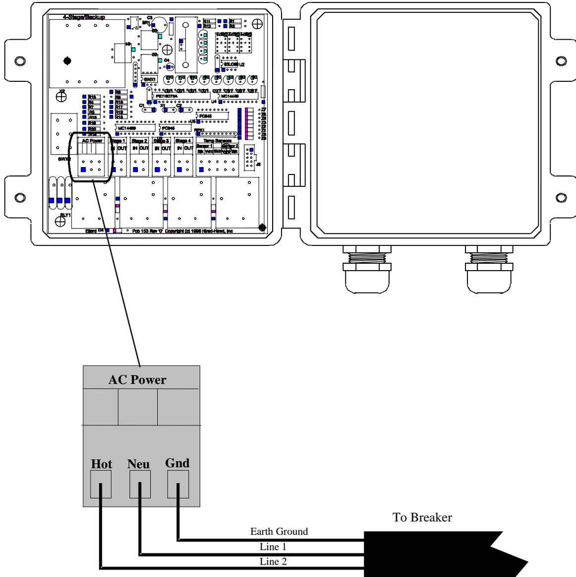
**Note: Make Sure that the SWX5 switch is set to the correct line voltage.**
