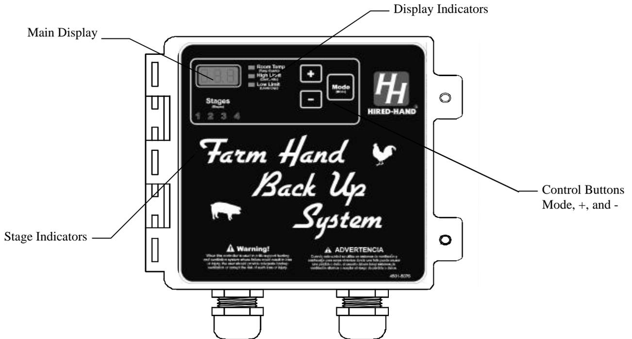
The Farm Hand Back Up System supplements a primary temperature controller such as a Farm Hand ST by providing auxiliary heat/cool stages and optional one room or two room temperature sensors. The Farm Hand Back Up can be set so that the High and Low Limits provide “back up” for a primary controller in the event of extreme variations from the target temperature or if the primary controller malfunctions.
